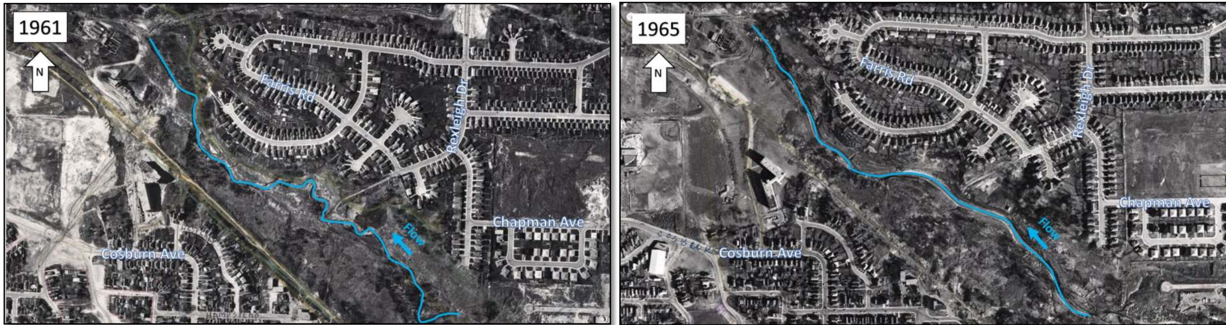
Taylor Massey Creek pre and post planform alteration in the 60s to accommodate sanitary sewer system.
