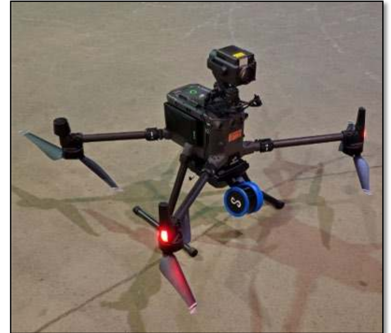
DJI Matrice 300 RTK equipped with AI capabilities for advanced autonomous flight
